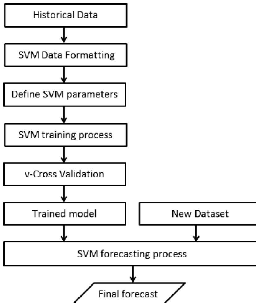
Fig. 4: Example of flowchart prediction in SVM
