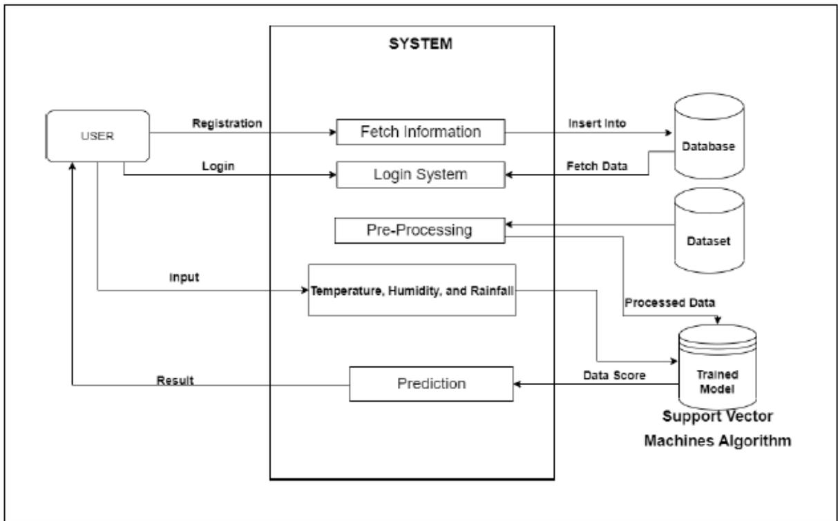
Fig. 11: The system architecture
